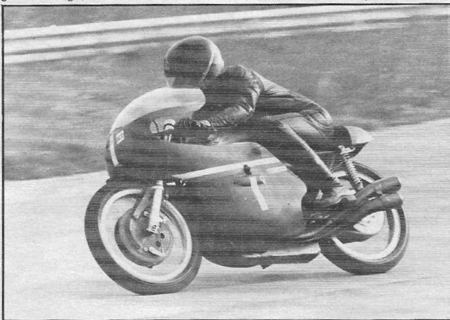
The machine's compact dimensions, based on a 50.5in wheelbase, are apparent in profile.
