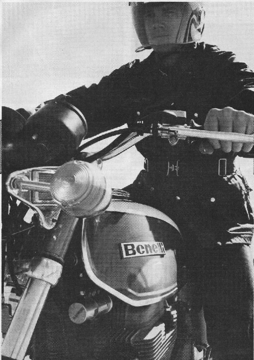
The engine sits low to the ground cradled by twin front downtubes. Note balance pipe between exhausts.
